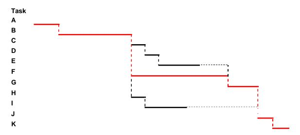
5 marks for correct structure and clear task dependencies, plus 3 for listing all tasks with some form of float (i.e. those in black above) and a further 2 for naming and highlighting (eg in red, as above) the critical path.
