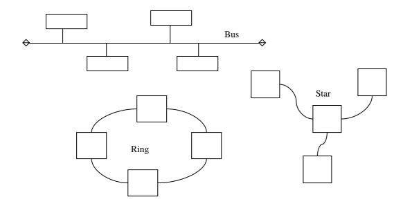
Bus – cheaper and easier to implement; limited in distance so suitable for LAN, slow because of possible collisions in sending messages; if one station fails does not affect the rest of the network.
