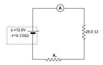
The diagram above shows an electrical circuit which consists of an unknown resistor  $R_x$  connected in series with a 25.0  $\Omega$  resistor and a battery of emf of 12.0 V and internal resistance 0.320  $\Omega$ . An ammeter connected in the circuit reads 200 mA.
