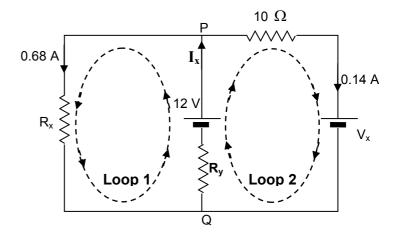
In the circuit shown above the unknown resistances  $R_x$  and  $R_y$  are equal. Use the nodes and loops marked to find:
