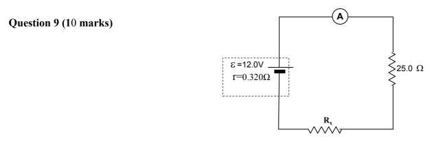
The diagram above shows an electrical circuit consists of an unknown resistor Rx connected in series with a 25.0  $\Omega$  resistor to a battery of emf of 12.0 V and internal resistance of 0.320  $\Omega$ . An ammeter connected in the circuit reads 200 mA.
