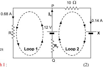
In the circuit shown above the unknown resistances  $R_x$  and  $R_y$  are equal. Use the nodes and loops marked to find:
