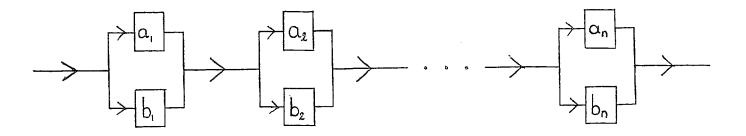
Assume that the 2n components  $(a_1, a_2, \ldots, a_n, b_1, b_2, \ldots, b_n)$  have a failure probability of 5% each, independently of each other. A block works if at least one of the two components in that block works. The circuit works if all blocks work.
