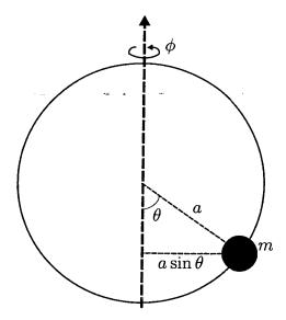
(b) A small bead of mass m slides freely on a smooth uniform circular wire of radius a. The wire is *free* to rotate about its vertical diameter and has moment of inertia of  $Ma^2/2$  about the rotation axis. Gravity acts downwards in the vertical direction with acceleration g. The system is described by two generalised coordinates  $\phi$  and  $\theta$  as shown in the figure, with  $0 \leq \theta \leq \pi$ .
