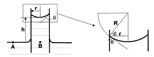
r is the radius of the capillary h is the height of the capillary rise R is the radius of the spherical surface of the liquid meniscus  $\theta$  is the contact angle of the liquid with the wall of the capillary
