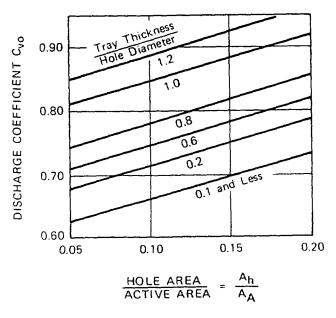
Discharge coefficient for sieve trays.
