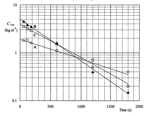
In each test, 10 kg of powdered solid was added to the agitated vessel containing 2 m<sup>-3</sup> of liquid. Liquid flowed in and out of the vessel at a rate of 4 L s<sup>-1</sup> and the concentration of solids in the outlet  $C_{out}$  was measured as a function of time.
