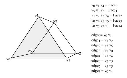
(b) Explain how the winged edge data structure would be completed - that is how the wings would be found. Give an example using edges 0 and 4.
