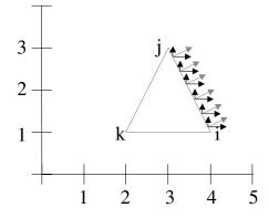
The finite element shown above has a thickness of  $\tau = 2$  mm. Its coefficient of thermal expansion is  $\alpha = 2*10^{-6} \, {}^{\circ}\text{C}^{-1}$  and the change in temperature is  $\Delta T = 50^{\circ}\text{C}$ . and the pressure acting on the surface (i,j) is P = 10 N/mm<sup>2</sup>. The element is of the plane stress type with
