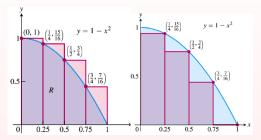
Approximate the area by calculating the sum of the areas of these rectangles f(c<sub>1</sub>)Δx + f(c<sub>2</sub>)Δx + ... + f(c<sub>n</sub>)Δx.
