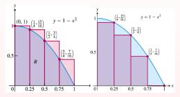
Approximate the area by calculating the sum of the areas of these rectangles  $f(c_1)\Delta x + f(c_2)\Delta x + \ldots + f(c_n)\Delta x$ .
