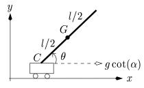
The length of the rod is l and at time t, CG makes an acute angle  $\theta$  with the x-direction. Given that the motion takes place in the xy-plane, where the y-axis is vertically upwards, use the equations of motion of the angular momentum of the rod about the point C to show that
