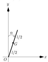
Calling the moment of inertia of the chimney about the axis Oz by I and assuming that the chimney remains in the xy-plane all the time and that at time t it makes the angle  $\alpha$  with the vertical, show that
