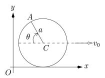
A is an arbitrary point on the circumference of the disc and  $\theta$  is the angle that the line AC makes with the horizontal, as shown in the diagram. Show that the magnitude of velocity of the point A is given by
