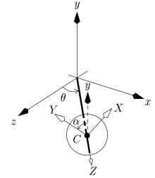
CX, CY and CZ are mutually perpendicular body axes, where CX and CY lie on the disc and CZ lies along the axis of the rod. At time  $t, \theta$  is the angle between the z-axis and CZ, and  $\alpha$  is the angle shown between upward vertical Cy and CY.
