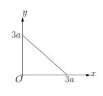
Obtain the Cartesian equations of the principal axes of inertia at the origin O for the lamina by considering its symmetry properties.
