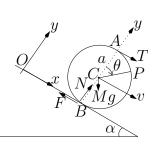
In addition to frictional, normal and gravitational forces, a thrust T, parallel to the positive x-axis, is applied at point A, as shown.
