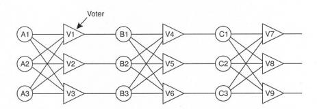
What is the maximal number of failed devices that the circuit given above can handle? 2 marks
