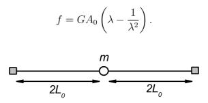
(b) Two light, thin pieces of rubber, of initial length  $L_0$  and initial cross sectional area  $A_0$  are attached by one end to a mass m and stretched to twice their initial length between clamps a distance  $4L_0$  apart, as shown in the above diagram. Assume the only force on the mass is due to the rubber.
