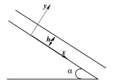
Defining Cartesian coordinates with x directed down the slope and y perpendicular to the slope and assuming from symmetry that the fluid velocity is of the form  $\mathbf{u} = (u(y), 0)$ , show that the x and y components of the momentum equation reduce to
