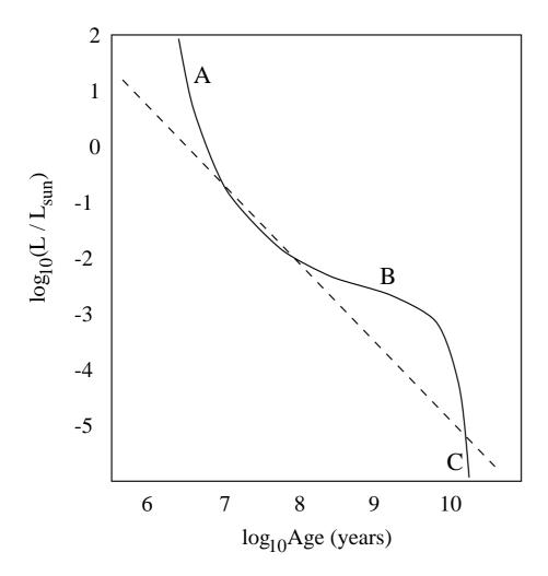
(b) The solid line in the above plot shows a cooling curve (luminosity versus time in logarithmic units) for a  $0.6 M_{\odot}$  white dwarf, constructed from a numerical model. The straight dashed line represents the cooling curve derived using the Mestel approach, which assumes completely degenerate electrons, an ideal gas of carbon ions, and energy losses from a thin atmosphere in radiative equilibrium.
