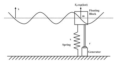
(i) The equation of motion for the vertical displacement  $\tilde{x}$  of the floating block is given by,
