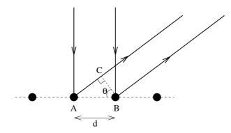
From the diagram, the path difference  $AC = d \sin \theta$ . Constructive interference occurs when AC is a whole number of wavelengths, and hence when
