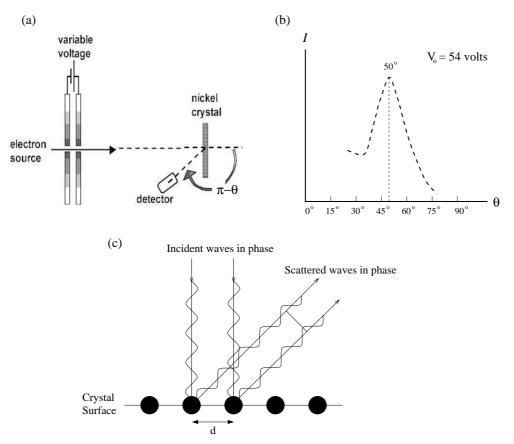
The Davisson-Germer experiment is shown in (a) above. Electrons are emitted from a heated filament, accelerated through a potential difference  $V_0$  volts, and directed at a crystal of nickel. When  $V_0$  is 54 volts, a peak in the signal I measured by the detector is observed when the angle  $\theta = 50^{\circ}$ , as in (b).
