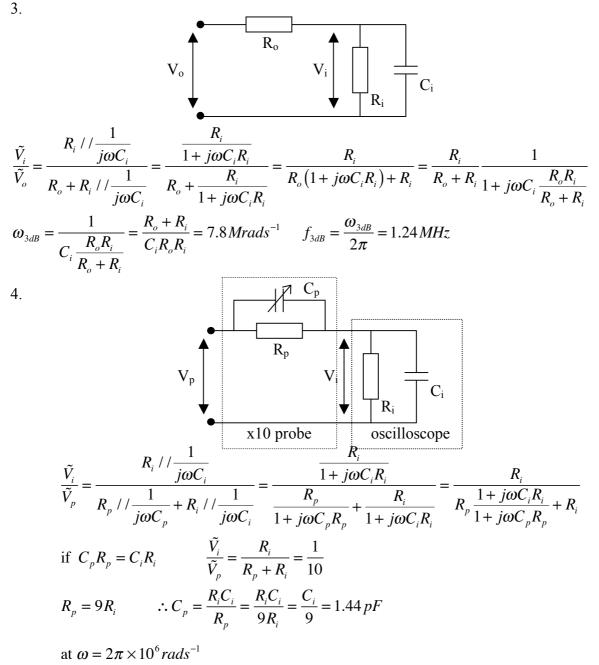
$$\left|Z_{C_{p}}\right| = \frac{1}{\omega C_{p}} = 110k\Omega \ll 9M\Omega$$
