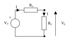
Power dissipated in the load  $P_L$  is given by
