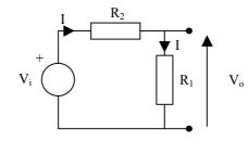
As no current is drawn and the output terminals the current in both resistors must be the same (I). By Kirchhoff's voltage law we can write
