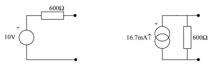
Input impedance of amplifier is  $20k\Omega$  so by a potential divider the voltage appearing at the output of the signal generator and the input to the amplifier is now
