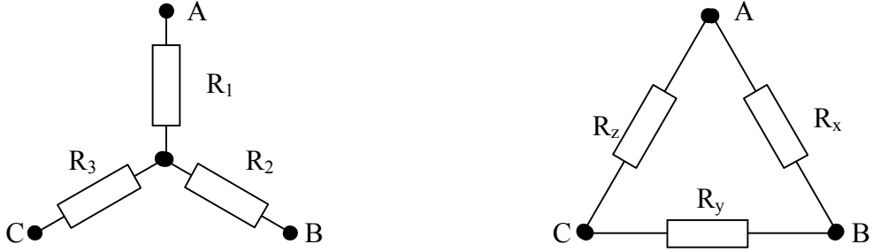
Figure 1 (a) Star formation of resistors (b) delta formation of resistors
