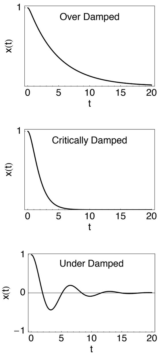
Figure 8.4: The three types of solution for a damped harmonic oscillator: over damped, critically damped, and under damped.
