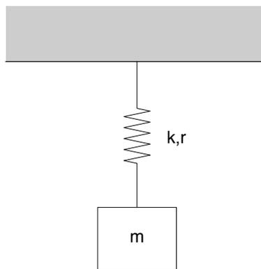
Figure 8.3: A harmonic oscillator consisting of a mass  $m$  attached to a spring of stiffness  $k$ , together with the forces acting on the mass.
