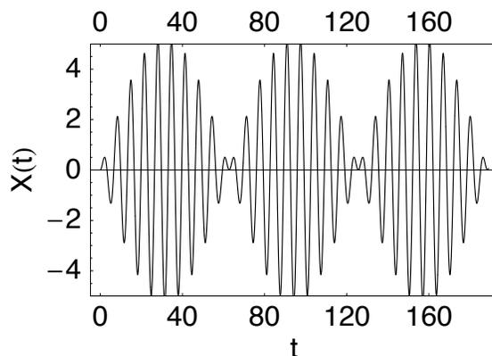
Figure 8.5: The quantity  $X(t) = mx(t)/2F_0$ , where  $x(t)$  is the solution in Eq. (8.86), for a undamped harmonic oscillator with a natural frequency  $\omega_0 = 1$  driven by a sinusoidal force with a frequency  $\omega = 0.9$ .
