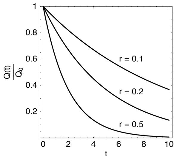
Figure 8.1: The solution in Eq. (8.16) plotted as  $Q(t)/Q_0$  against  $t$  for three values of the rate constant  $r$ . With increasing  $r$ , the amount of material at time  $t$  decreases substantially.
