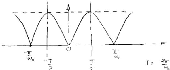
$$C_R = \frac{1}{T} \int_{-\frac{T}{2}}^{\frac{T}{2}} x(t) e^{-jk\omega_0 t} dt = \frac{1}{T} \int_0^T -\sin \omega_0 t e^{-jk\omega_0 t} dt + \frac{1}{T} \int_0^T \sin \omega_0 t e^{-jk\omega_0 t} dt$$
