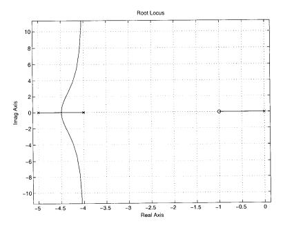
angles of the asymptotes are  $\sigma = -4 \& \psi = \pm 90^{\circ}$ . For the real axis intercepts, we search for real roots of  $\frac{d}{ds}K(s)G(s) = 0$  or  $s^3 + 6s^2 + 9s + 10 = 0$ , which has a real root at  $\boxed{-4.492}$  according to the hint in the question.
