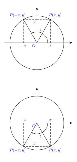
Using these two diagrams we can see that for any y with -1 < y < 1 there are two solutions to  $\sin \theta = y$  with  $\theta \in (-\pi, \pi]$ .
