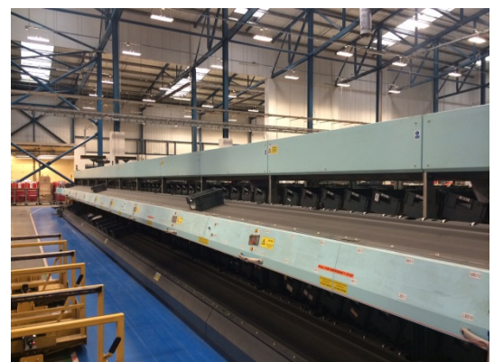
Mail Trays on FSM conveyor at Leeds Mail Centre
