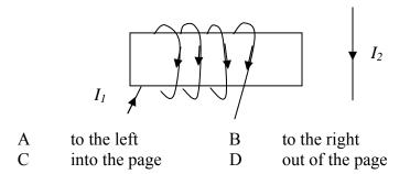
A solenoid, of length *l* closely and uniformly wound as shown, carries a steady direct current. A search coil is placed at different positions along the solenoid.
