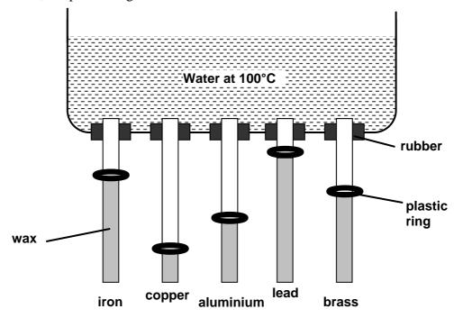
Complete the table below by placing the five conductors in the above diagram in order of conductivity putting the best conductor first.
