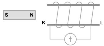
When the magnet is pushed into the coil, the **galvanometer pointer** deflects **clockwise**.
