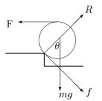
Let the angle between the radius to the point of contact with the step and the downward vertical be  $\theta$ , as shown.
