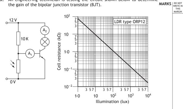
(a) Determine the light level to fully saturate the transistor. Refer to the graph shown, which shows how the resistance of the LDR responds to light level. Assume  $V_{BE} = 0.7 V$ .
