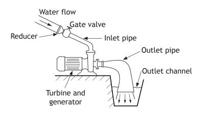
The engineer measured the electrical output from the generator to be 22A at 230 V. The mass of water flowing through the inlet pipe into the generator was 2500 kg every second at an average flow rate of  $3 \cdot 2 \text{ ms}^{-1}$ .
