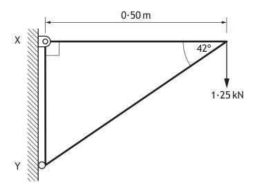
Calculate the magnitude and direction of the reaction at Y.
