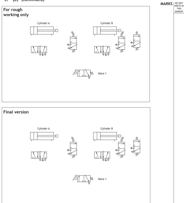
(ii) As a safety feature, the designer of the machine decided to add an extra valve to the circuit. In this new system, two valves have to be actuated together for the sequence to start, producing AND control. Add the valve and actuators to your circuit diagram above and connect it to the rest of the circuit to produce this type of control.
