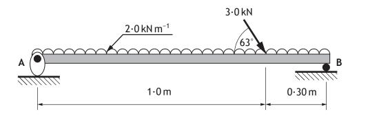
(d) Determine the magnitude and direction of the reaction at A.
