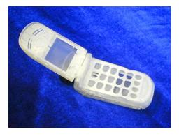
Rapid prototype of a mobile phone casing
