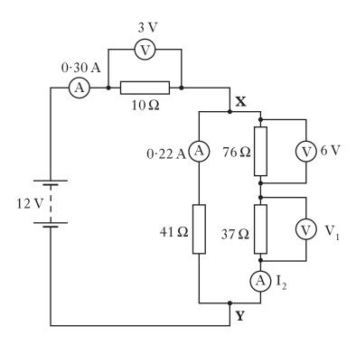
(a) (i) Calculate the overall resistance between points **X** and **Y**.
