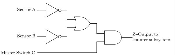
(a) Complete the Boolean expression for Z in terms of A, B and C, with reference to the logic diagram above.
