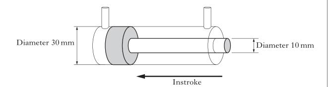
(d) Calculate the **instroking** force produced by the cylinder.
