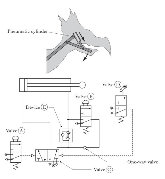
The dragon's mouth is operated by pressing Valve (A), or by pressing Valve (A) and (B) together.
