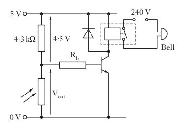
(a) Calculate the resistance of the LDR when  $V_{out}$  is  $0.5 \, V$ .
