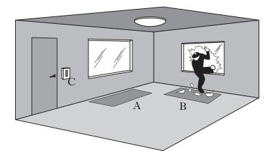
A buzzer will sound if master switch **C** is on and either pressure switch **A** or **B** is also pressed.
