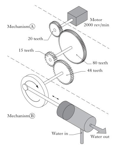
The system consists of **two** separate mechanisms.
