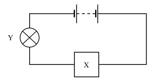
X is used to vary the brightness of bulb Y. What is component X?
