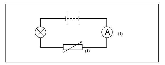
(d) The voltage of the battery in the circuit is 6 volts. The ammeter shows a current of 0.1 amperes. Calculate the resistance of the circuit.
