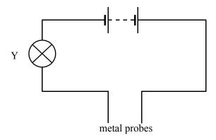
(a) The student touches the metal probes together and bulb Y lights.
