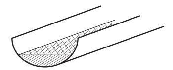
The cross-section of the guttering is a semi-circle with diameter 10 centimetres.
