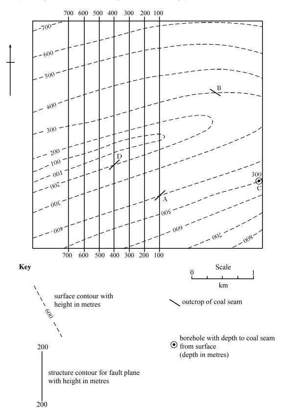
Marks Structure contours have already been drawn for a fault plane which crosses this area. **(a)** Draw in the outcrop of the fault plane, remembering that the fault will outcrop where relief contours cross structure contours of the same height. 700 600 500 400 300 200 100 -700-600 Ν 500 В 400 300 200 100  $\iota_{00}$ 300 002 T 005 *p*02 - 00<sup>4</sup>. 009 *00* L 700 600 500 400 300 200 100 Scale 0 1
