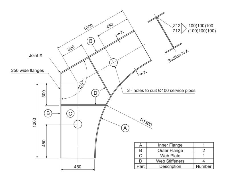
Figure 1 Note: All plates 10 mm thick
