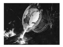
For the health and safety of the workers in the factory, it is important that the ladle is full but does not overflow. The volume of a ladle reduces each time it is used since steel not fully drained away will solidify in the ladle.
