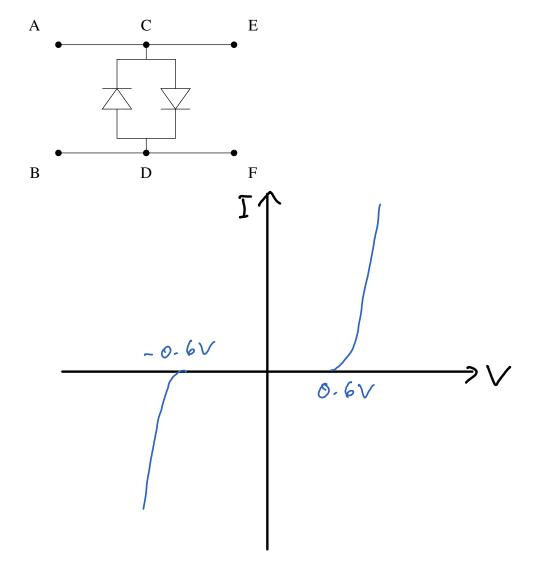
For small signals (low voltage), current doesn't flow through C-D. Amplifier operates.
