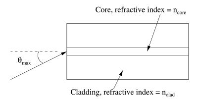
Light may only be transmitted along the fibre if the incident angle of the light is less than a maximum angle  $\theta_{max}$ . By using your equation from above and Snell's Law, or otherwise, derive an expression for  $\theta_{max}$  in terms of the core and cladding refractive indices only.
