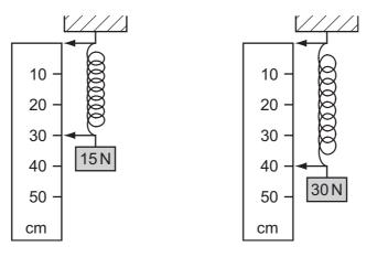
When the weights are removed, the spring returns to its original length.
