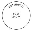
Which current is needed to light the bulb at normal brightness?
