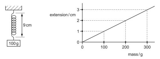
What is the length of the spring after the 100 g mass has been removed?
