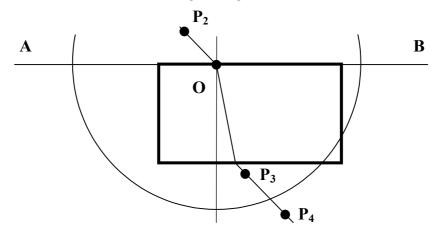
Measure and record the angle of refraction,  $\mathbf{r}$ , of the ray as it enters the glass block.
