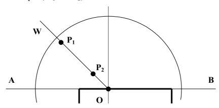
Measure and record the angle of incidence the ray **WO** makes with the normal to the glass block.
