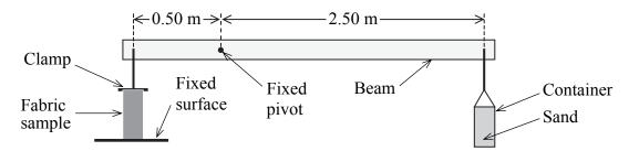
(a) The force applied by the sand and container is 60 N. Calculate the moment of this
