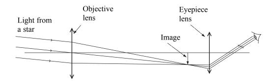
(a) Parallel rays of light from a distant star are refracted by the objective lens to form an image as shown.
