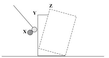
For the chain reaction to continue the block of wood must topple over completely.
