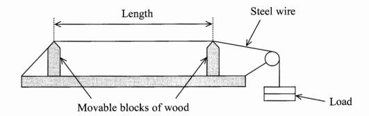
When the wire is plucked at its centre it moves rapidly as shown below. The length of the wire represents half the **wavelength** of the vibration.
