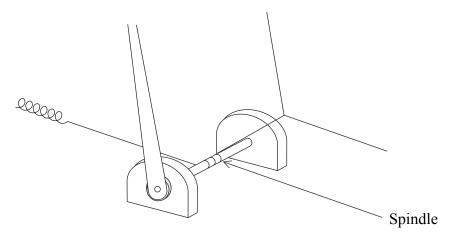
Some thread is wrapped around the pointer spindle. When there is current in the wire PQ the point R is pulled down by the spring and the pointer then moves over the scale.
