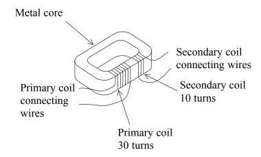
(a) The diagram shows two insulated copper wire coils wound onto a metal core to make a simple transformer.
