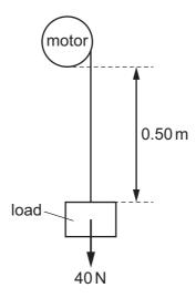
The load weighs 40 N. The power of the motor is 20 W and the system is 25% efficient.
